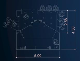
TOTAL AREA REQUIRED: 18.8 m2 ELECTRICAL DEMAND: 380V TRIPLE (3F +1N +1PE) - 13.52kVA
