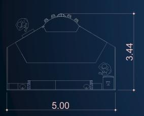
TOTAL AREA REQUIRED: 18.8 m2 ELECTRICAL DEMAND: 380V TRIPLE (3F +1N +1PE) - 13.52kVA
